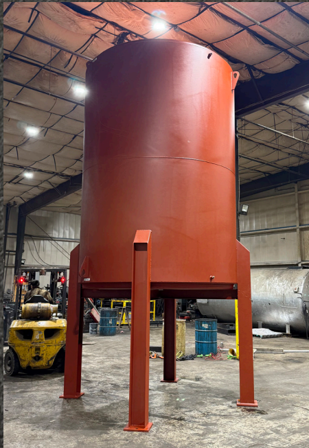
4,500 GALLON COOLING TANK
